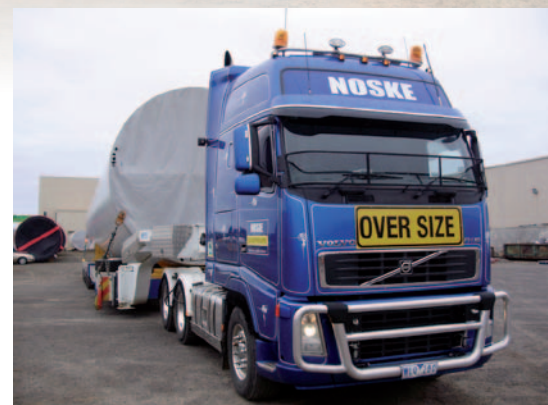
A tower section is loaded and secured on a specialised trailer, ready for delivery to the jobsite.
